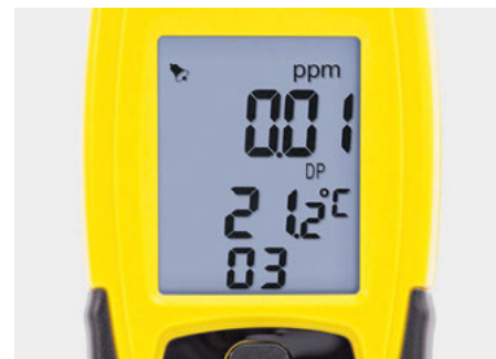
The backlit LCD display of the OZ-ONE simultaneously indicates two parameters that can also be read in poorly illuminated surroundings.
