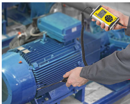
The structure-borne sound probe with stainless steel tip is ideally suited for non-destructive testing, e.g. to check rotating machine components for bearing wear.
